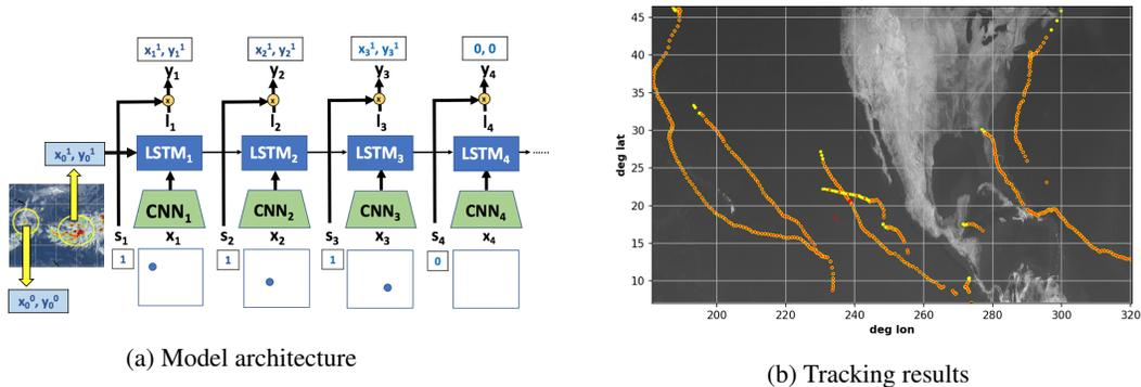
Figure 1: (a) Model: Given the initial position of the target trajectory, the model predicts the remaining positions at each time step. (b) Tracking results: Comparison between ground-truth (yellow) and model prediction (red).
