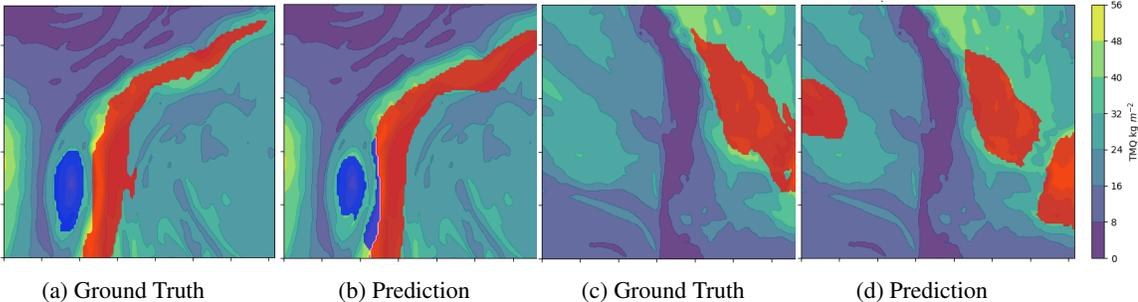
Figure 3: (a) Sample cropped ground truth image with AR delineated in red and TC delineated in blue. (b) Corresponding (to Fig.3a) sample cropped predicted image, with AR in red and TC in blue. (c) Sample cropped ground truth image (d) Model prediction for Figure 3c. Here the model fails to isolate the AR on the right side as a contiguous region, and it finds a false positive for an AR on the left side. These errors may have been introduced when cropping global images.
